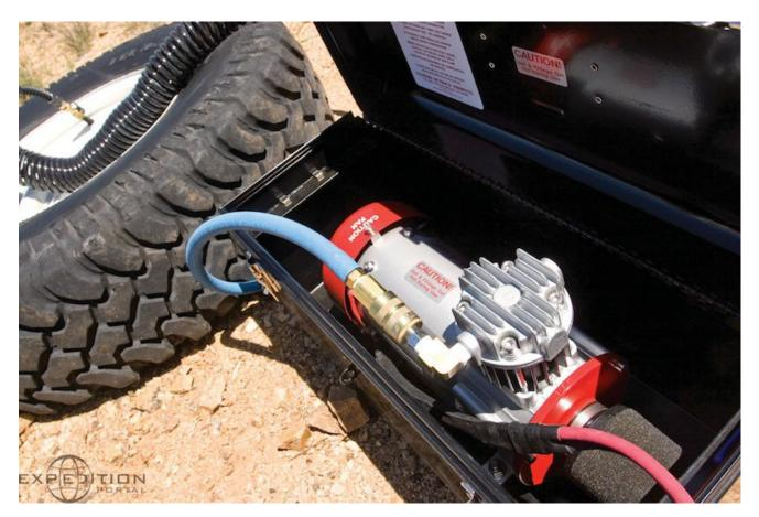
The moment you open the steel tool box encasing the ExtremeAire Magnum Portable, it's obvious you're looking at a product with a lot of thought behind it. The hose connections are protected with spring coils, the leads to the stout, 4-gauge battery cables are sealed and shrink- wrapped, and a fat, washable, oiled UNI-filter protects the intake of the compressor, which is powered by a massive, fan-cooled, 1 1/2-horsepower motor. Magnets at each end of the box hold a tire gauge and LED penlight.
