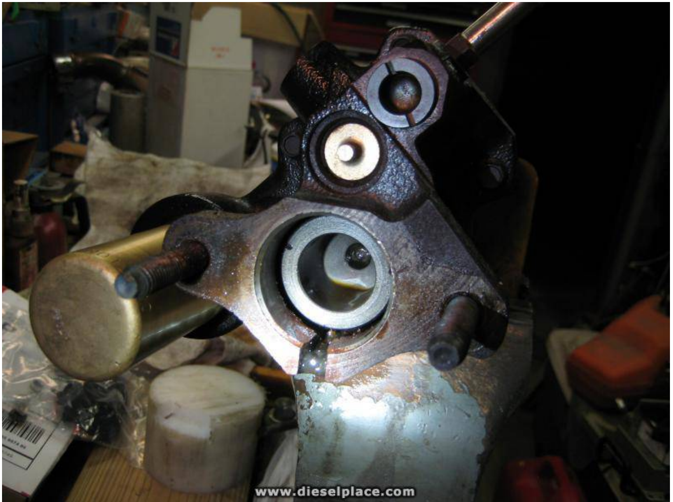
Pic 2 PS fluid after spider removal and MC actuator rod
