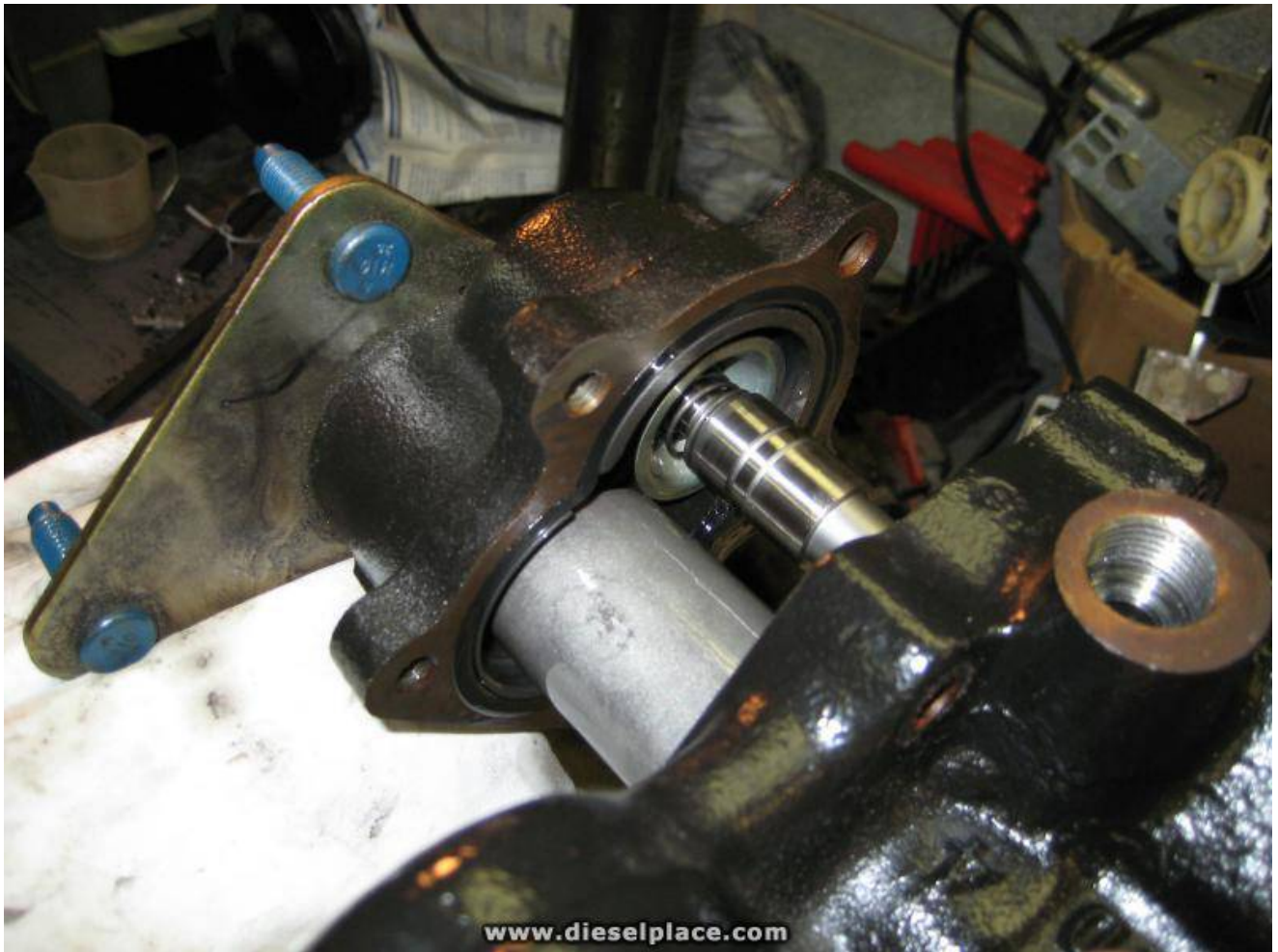
Pic 6 power Hydro halves coming apart.
