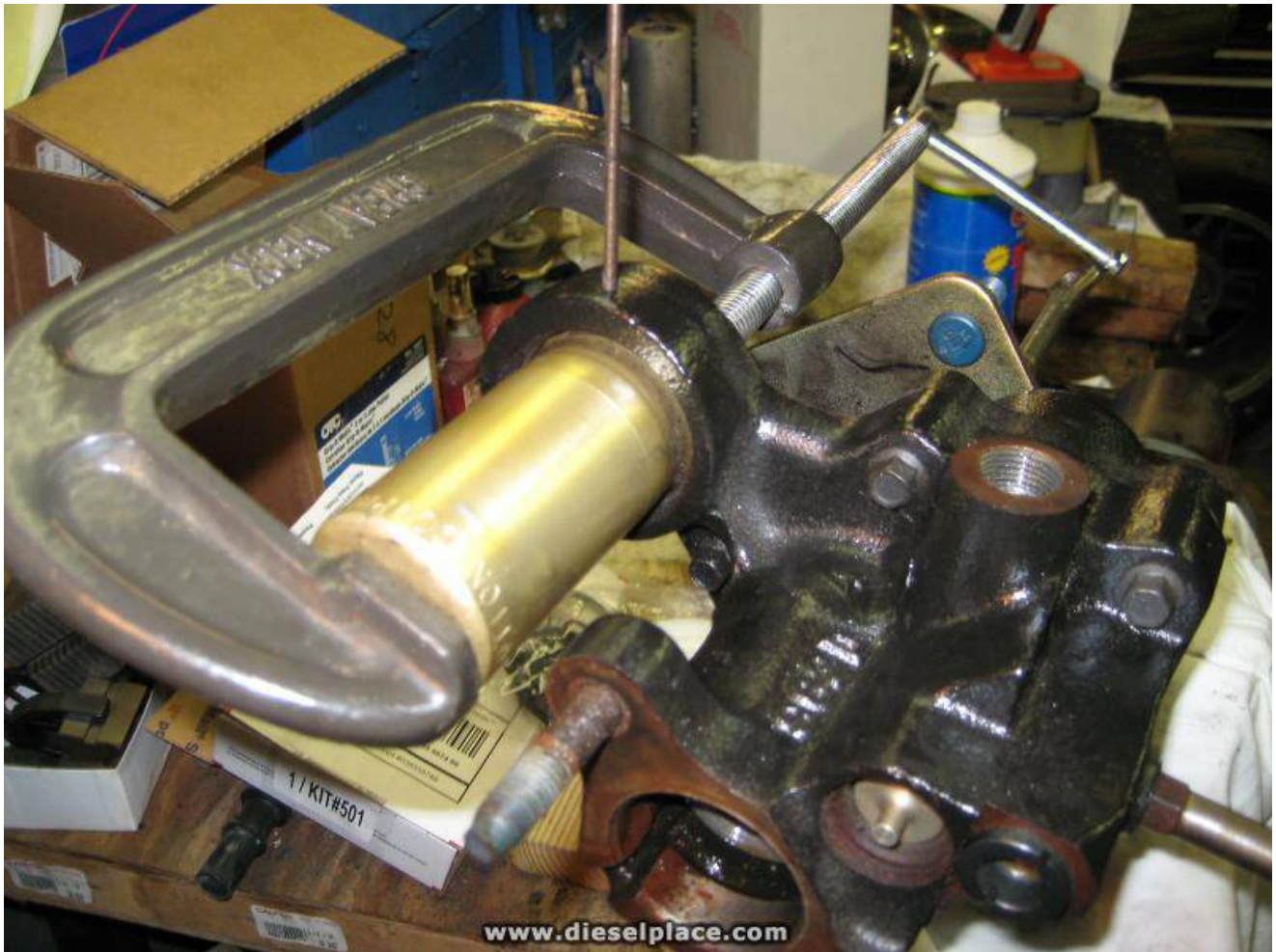
Pic 3 Removing the accumulator (note 1/8 pin punch to remove snap ring)
