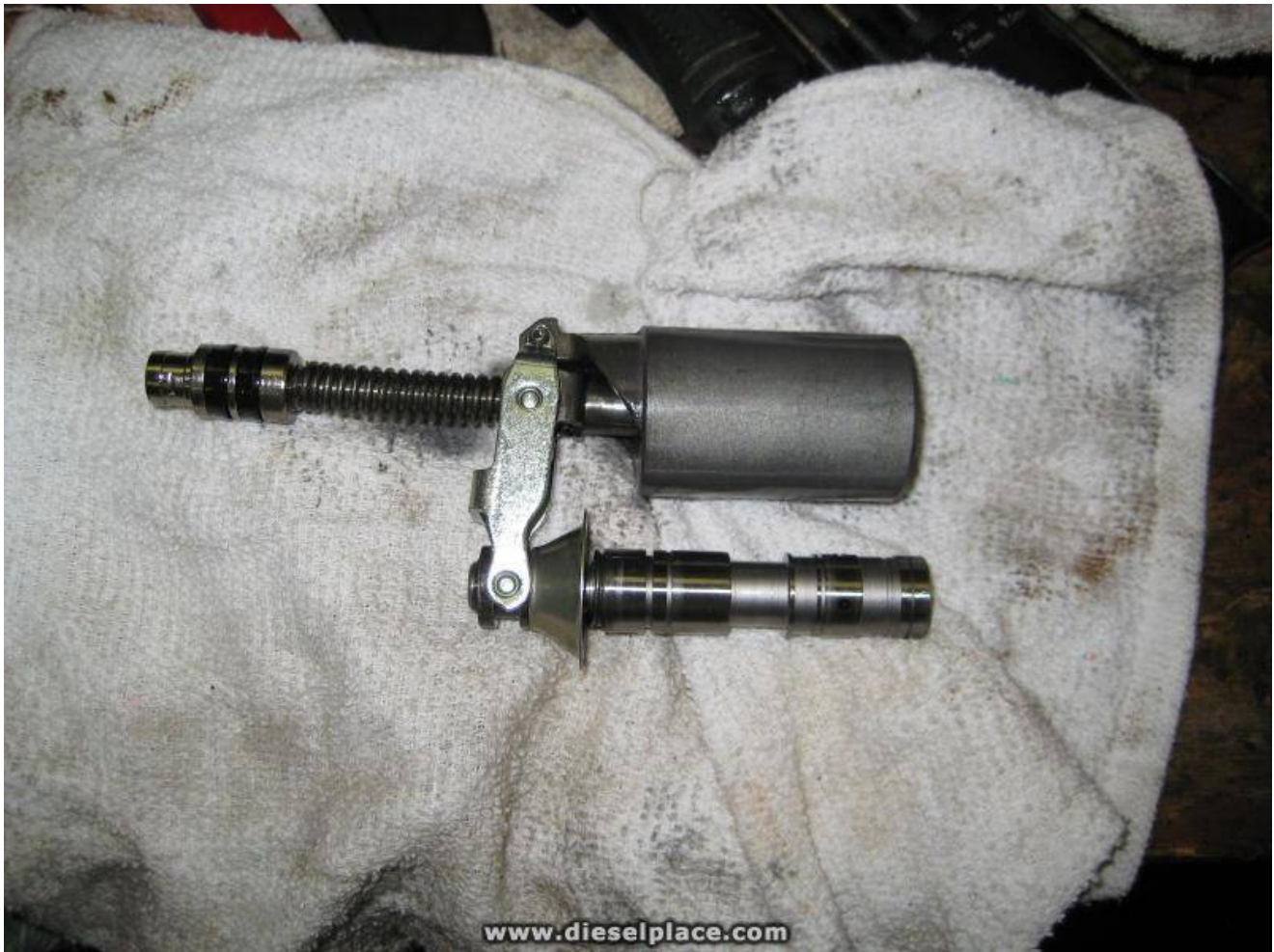
Pic 7 Push rod /Power Piston assembly w/ spool valve.
