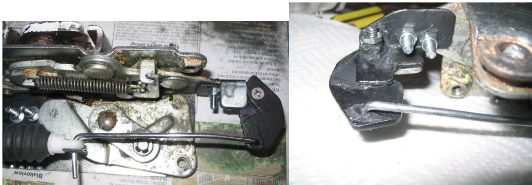
Figure 2 Moving Plate System (Locked) Note the moving plates were enlarged a bit after these photos was taken to increase the area the pusher had to push against. It was too close to the edge in this design.
