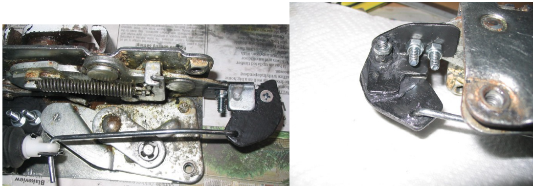
Figure 1 Moving Plate System (Unlocked Position)
