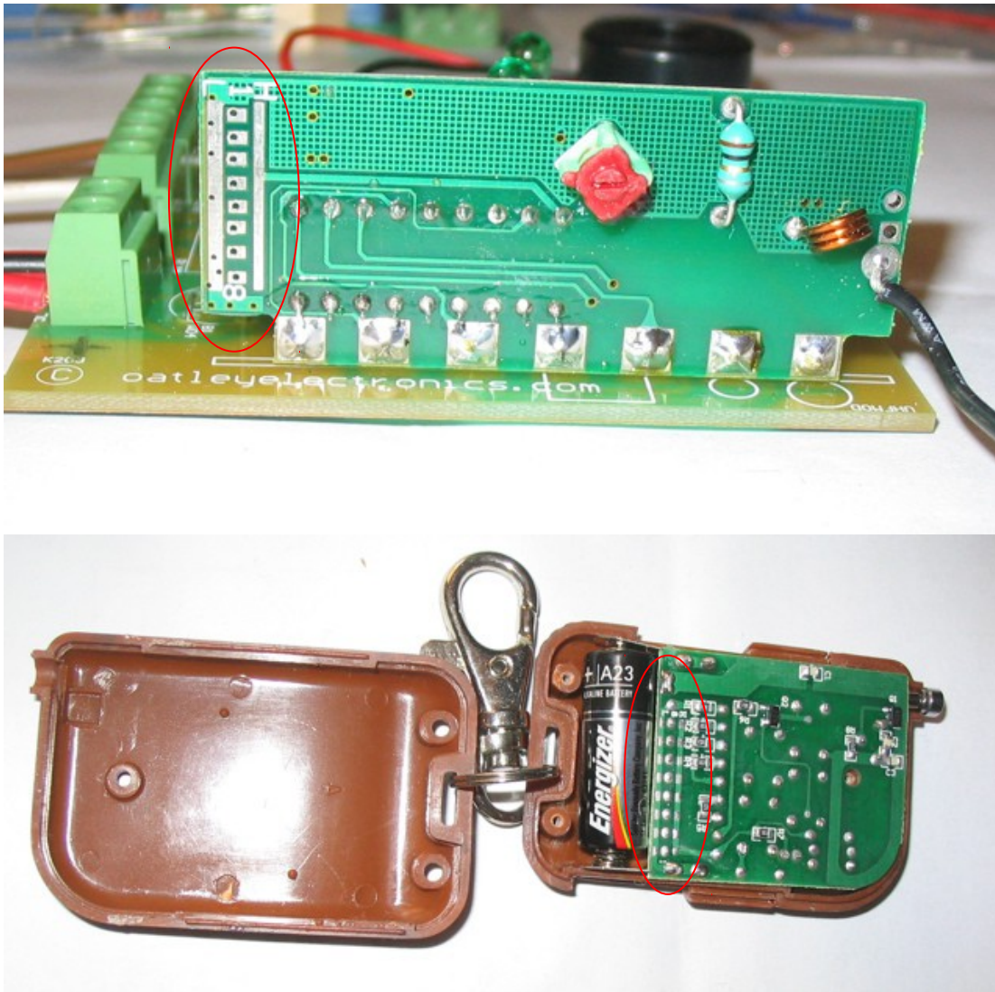
Figure 18 Encoding Connection Areas on receiver and Transmitter circuits. Both must be wired the same.
