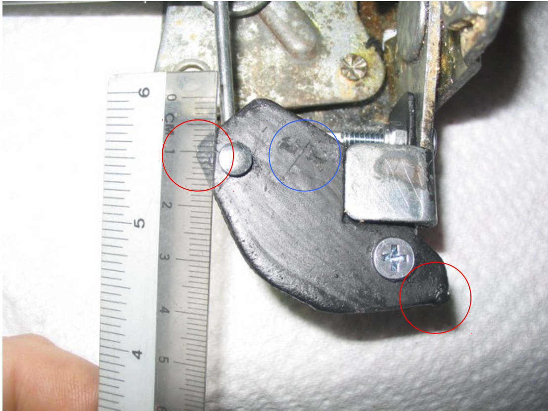
Figure 7 Moving plate showing ruler for scaling. Note, this is an enlarged moving plate from those shown in Figs 1 and 2. Subsequently, I had to grind off the corners (left and right as shown in red) so it didn't foul the door frame and window slide in operation. The area where the pusher hits can just be seen (in blue) and shows why I had to enlarge it, it was very close to the edge.
