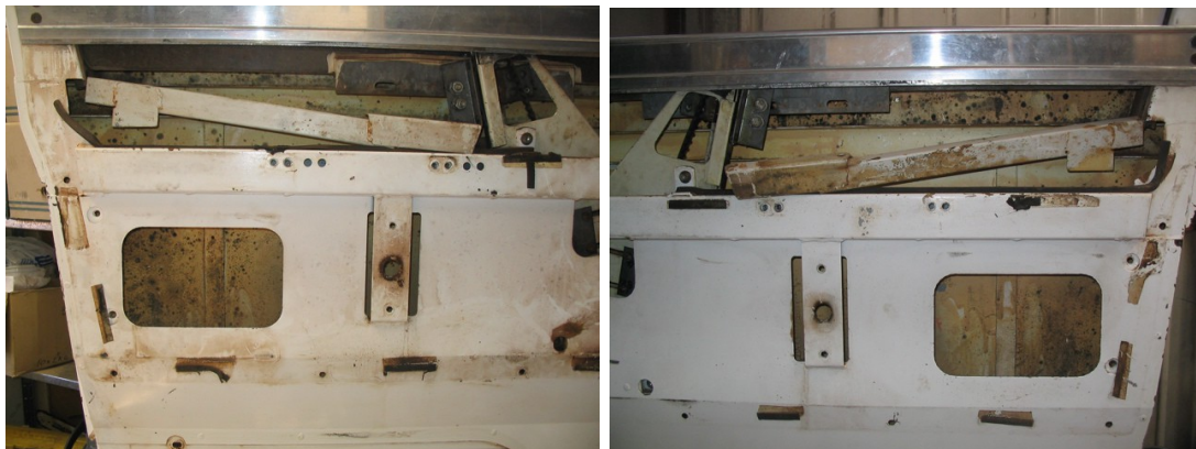
Figure 8 Shows Window Slides relocated to enable catch mechanism to be removed
